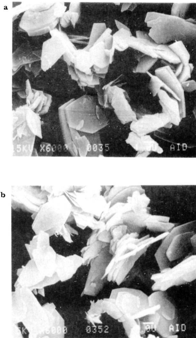
Figure 7. SEM photomicrographs of (a) \text{VO}(\text{HPO}_4)\cdot 0.5\text{H}_2\text{O} and (b) (\text{VO})_2\text{P}_2\text{O}_7 produced from it. The bar in the lower right corresponds to 1\ \mu\text{m} .
